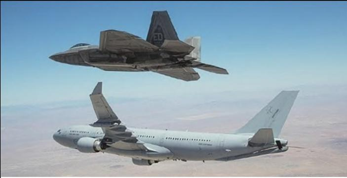
REFUELLING trials with the US Air Force (USAF) will clear No. 33 Squadron's KC-30A Multi-Role Tanker Transport aircraft to work with the advanced F-22 Raptor fighter. Eight test flights between the two aircraft were conducted from Edwards Air Force Base in California in August and September. The data is now being assessed to complete the standard procedures for refuelling activities involving both aircraft. Serving as an air dominance
